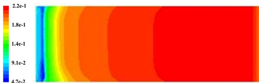
Fig. 6. Liquid water saturation in cathode catalyst layer.
